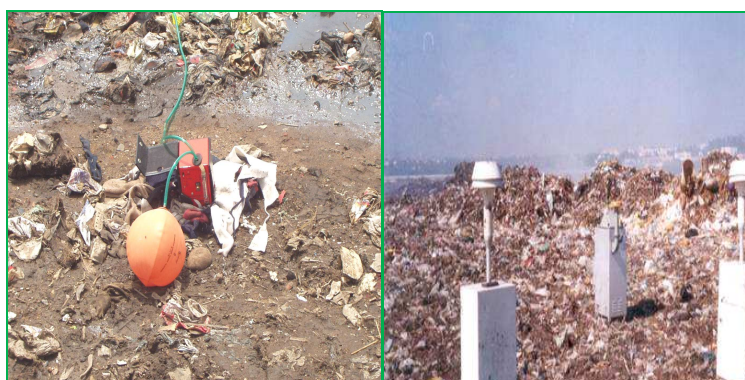
Fig. 2: Air Sampling approaches in Open Dumpsites for Vocs and Particulate Matter Characterization
