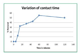
From the graph, it is evident that the %removal increases with increase in contact time. The optimum time for the removal of  $NO_2$  is 60 minutes. The percentage removal of  $NO_2$  increases with the increase in contact time and it follows a smooth curve which indicates that the process is of first order (Zhe Ming et al (2004)).
