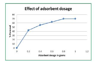
From the graph, it is clear that the % removal increases with increase in adsorbent dosage. Greater the number of adsorbent sites, greater is the percentage of adsorption (Zhang et al. 1993).
