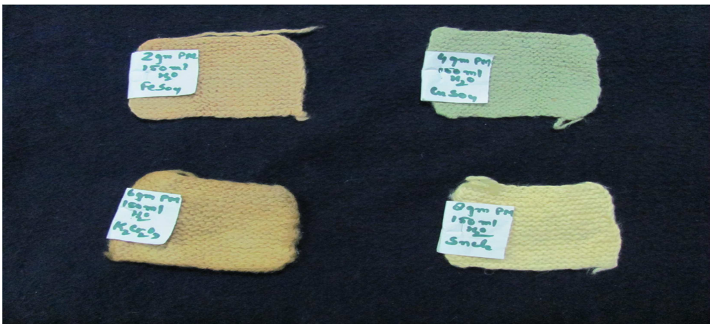
Fig. 4. Dyed samples for Simultaneous Mordanting method followed by four different Chemical Mordants with few drops of lemon juice as Natural Mordant
