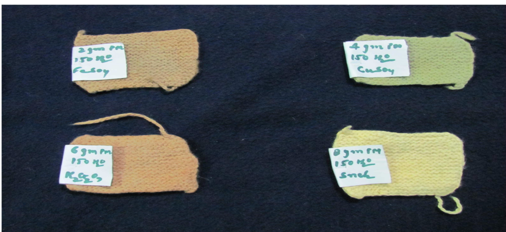
Fig. 5. Dyed samples for Post-Mordanting method followed by four different Chemical Mordants with few drops of lemon juice as Natural Mordant
