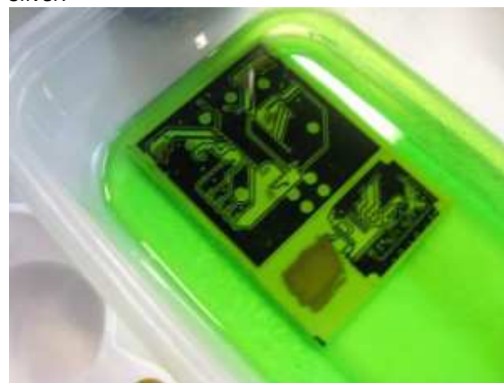
Dissolved copper in the acid bath turned the solution green (By Brad 2011).
