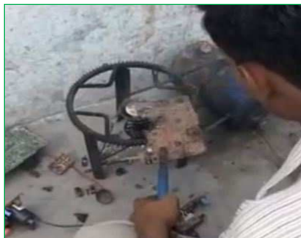
A worker burning circuit board to get metals in Seelampur, India. (Keekeesocean uploaded on 2012).
