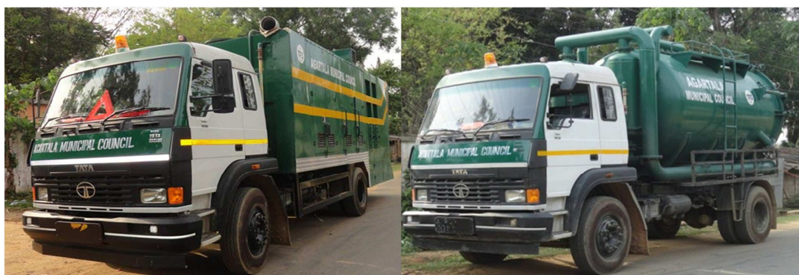
Fig. 5: Covered modern trucks used for waste transportation and other waste disposal process
