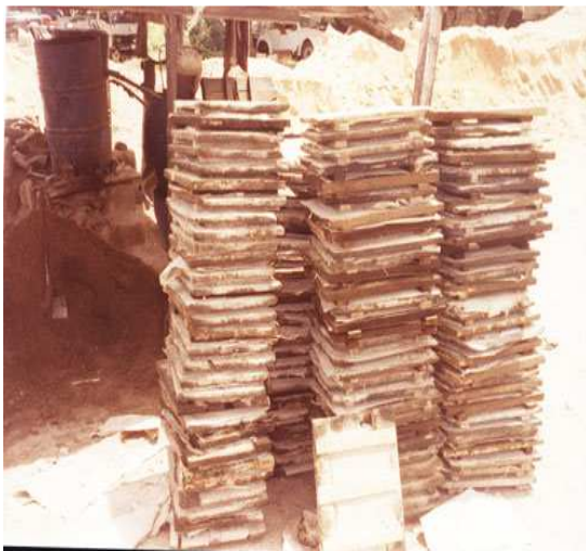
Figure 2.3: Pallets treated with used oil in block making
