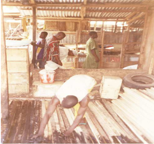
Figure 2.2: Application of used oil to wood treatment
